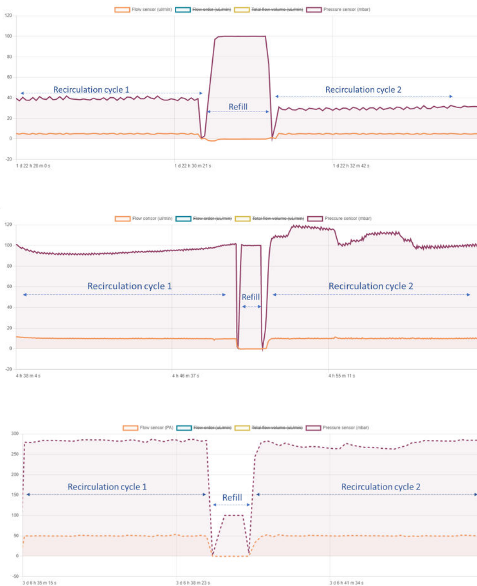
Figure 10: Flow rate and Pressure rate monitoring over time for 5 \mu\text{L}/\text{min} , 10 \mu\text{L}/\text{min} or 50 \mu\text{L}/\text{min} , respectively.
