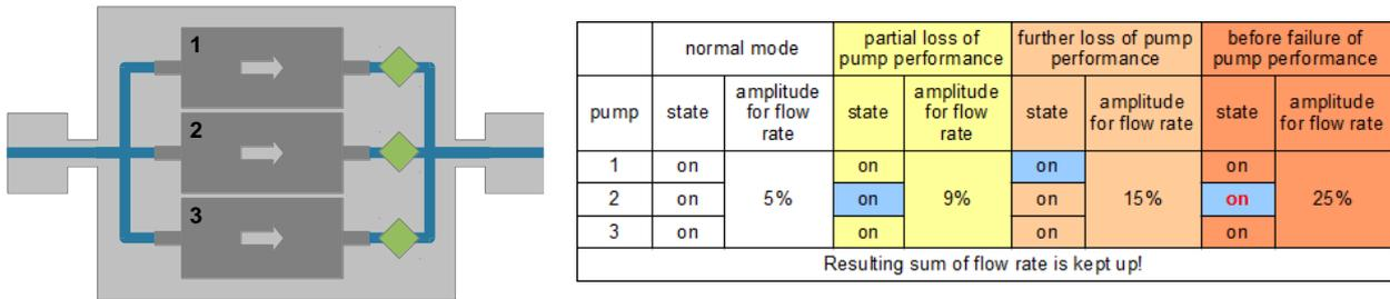
Figure 5: Parallel control of three pumps with one amplitude for all.
