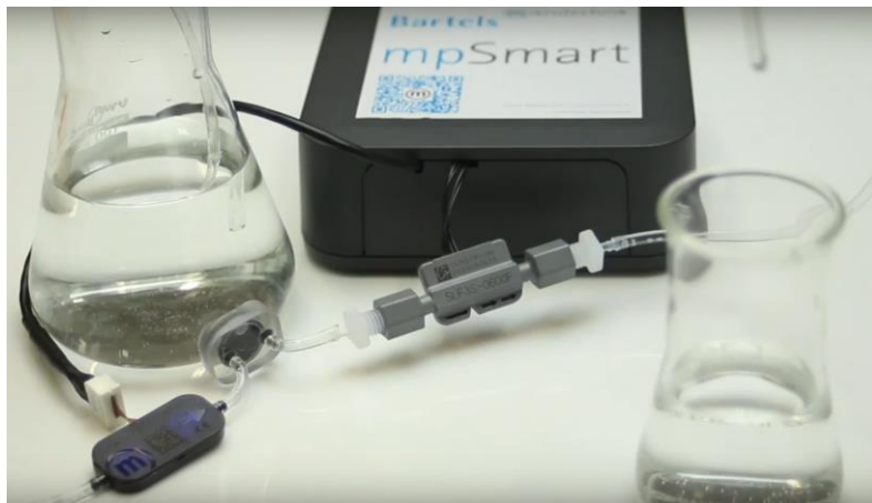
Figure 5: Typical set-up for the application of the mpSmart Dosing.
