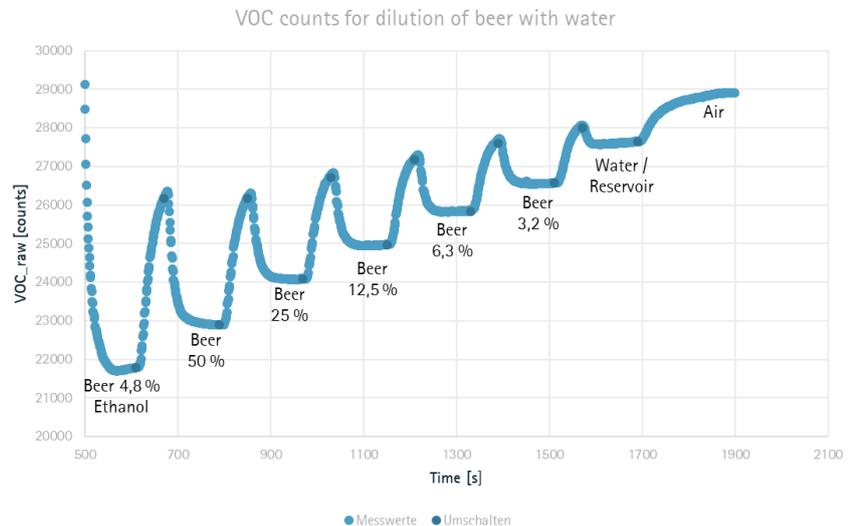
In conclusion, CO<sub>2</sub> as well as VOC concentrations rise with advanced fermentation. That way, by simply assigning a reference (e.g. beer with 4.8% C<sub>2</sub>H<sub>5</sub>OH), the fermentation process of yeast into beer can be protocolled industrially with very little space and resources needed. Since all data can be obtained via gas phase analysis, contaminants are mostly excluded from the measurement.
